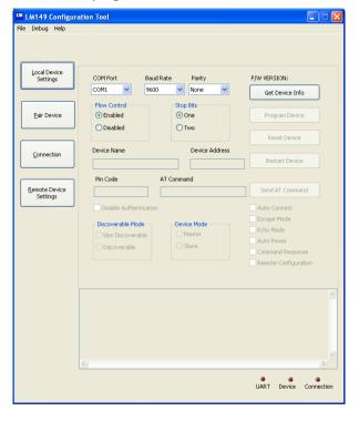
The LM058 can also be paired via the configuration program using the "pair Device" button. It takes you to the page which provides option for pairing/Unpairing adapters.
